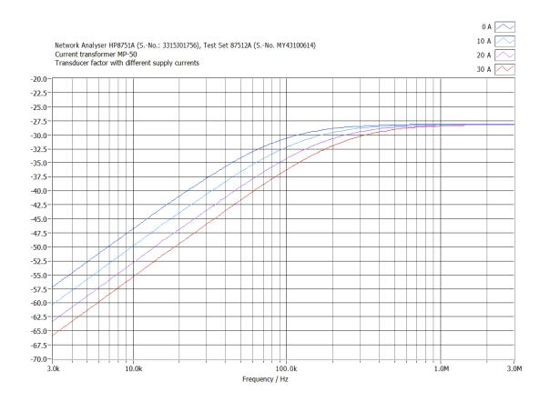
The MP-50 current monitoring probe measures RF common mode currents (asymmetrical currents) on single conductors or conductor bundles. Depending on the low frequency current saturation effects may occur, which shift the lower frequency characteristics to somewhat higher frequencies.
